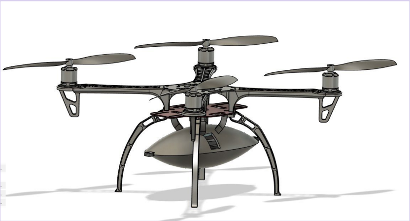
FIG 09 - TEST AIRFRAME WITH RELAY RECEIVER AND AVIONICS
