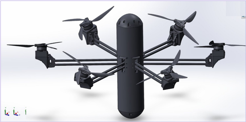
FIG 01 – AIRFRAME IN THE EXTENDED (AIR) CONFIGURATION
